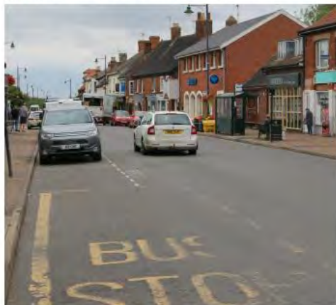
2.6 The lack of dropped curbs limits accessibility for those using wheelchairs and mobility scooters, and can force them to use the road rather than the pavement
