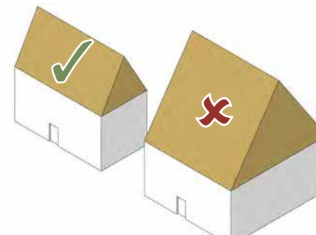
Steep roof pitches on deep floorplans create bulky buildings and roofs that are intrusive in the street scene and a poor reflection of local character.
