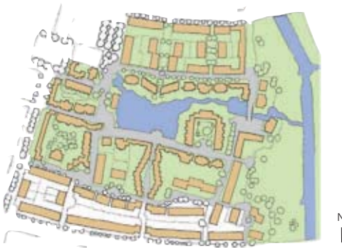
Ecolonia's layout is centred on a reed-fringed pond, with buildings orientated to maximise solar gain
