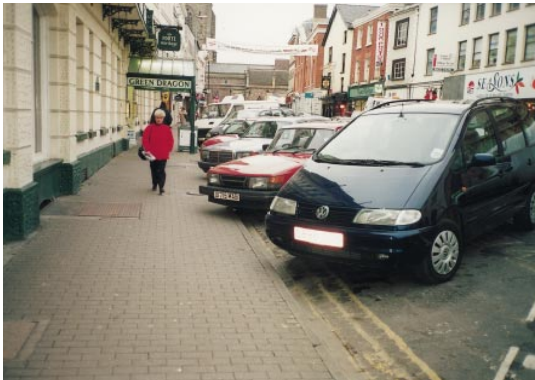
Chevron parking tends to lead to vehicles overhanging the footway. Courtesy: Ove Arup/David Davies.
