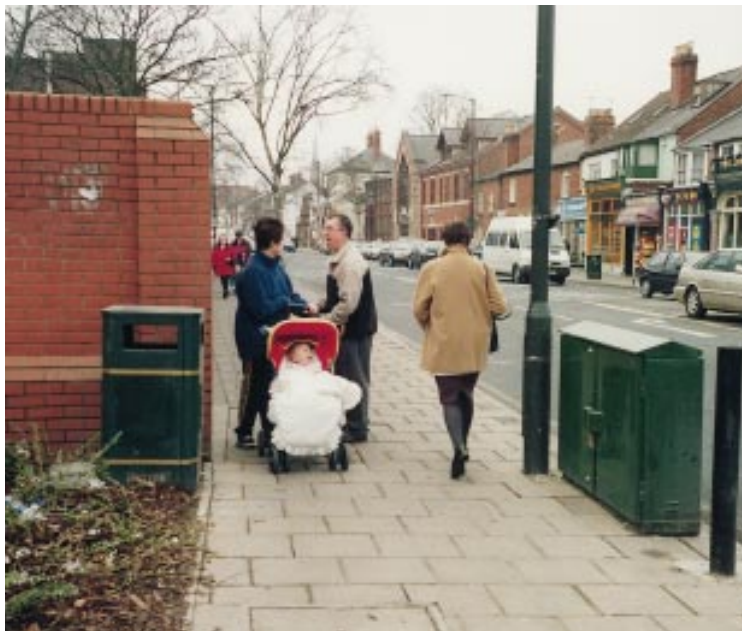
Well-positioned street furniture maximises the usable space for pedestrians. Courtesy: Ove Arup/David Davies.
