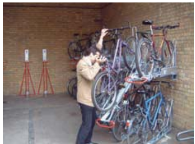
Figure 11.6 Spring-assisted stacking cycle rack (Tony Russell CTC)
