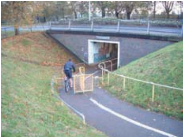
Figure 8.10 Barrier to reduce speed on approach to subway (CTC Benchmarking)
