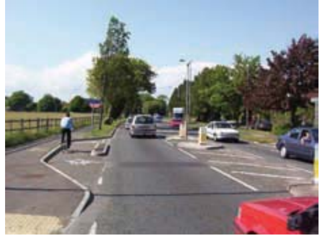
Figure 10.4 Jug-handle turning at busy non-priority crossing (Patrick Lingwood)
