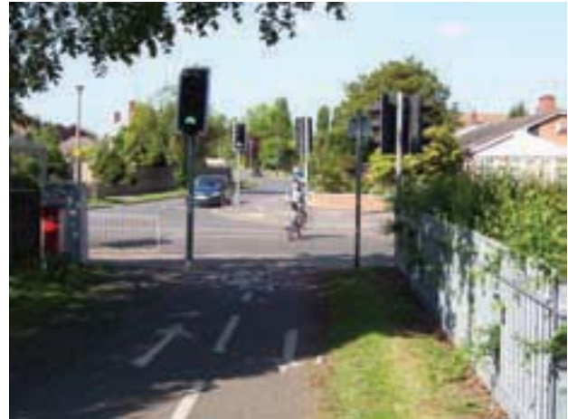
Figure 10.7 Traffic light at end of cycle track (Rob Marshall)
