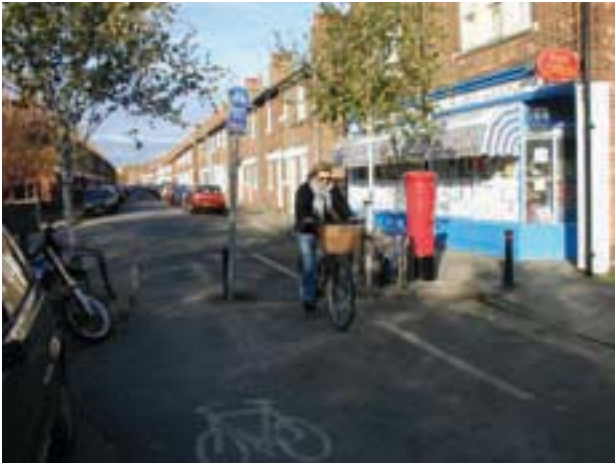
Figure 4.2 Mid-link road closure with cycle access (Patrick Lingwood)
