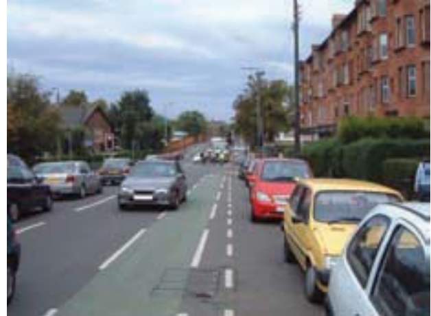
Figure 7.5 Cycle lane with buffer zone alongside parking bays, Glasgow (Tony Russell)
