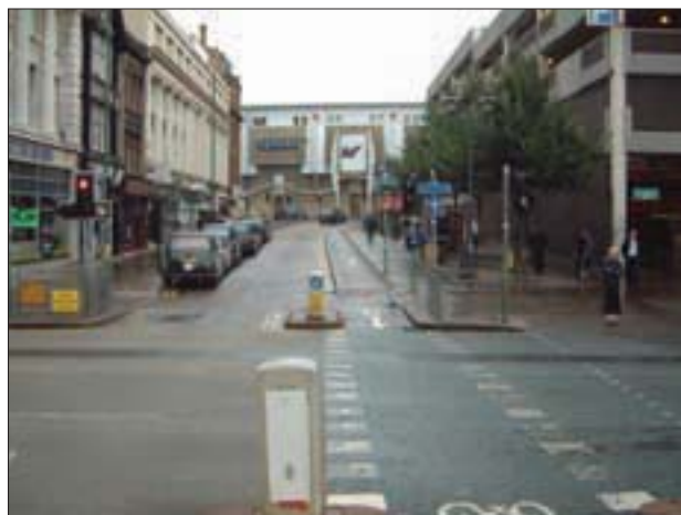
Figure 9.3 Elephants' feet markings, (CTC Benchmarking)
